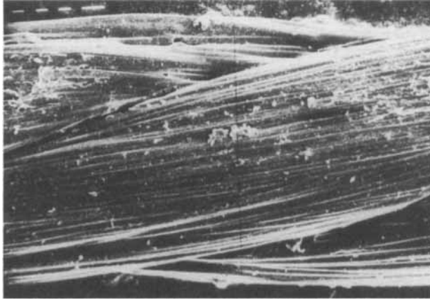
FIGURE 2 SEM photomicrograph of a chemically treated polyester cord (40 \times ).
