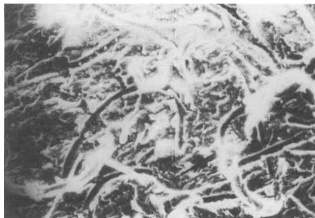
FIGURE 15 SEM photomicrograph of abraded surface of mix B with ploughing marks and disintegrated fibers (40 \times ).
