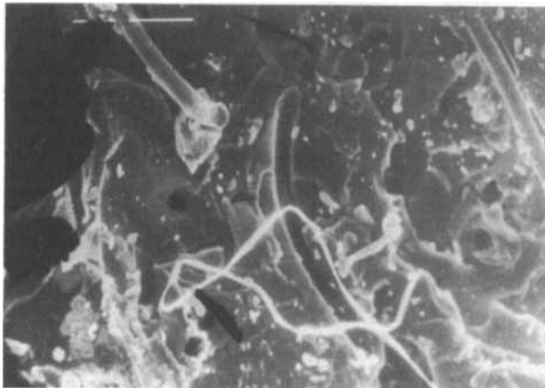
FIGURE 7 SEM photomicrograph of tensile fracture surface of 10 phr loaded fibers in transverse orientation (100 \times ).
